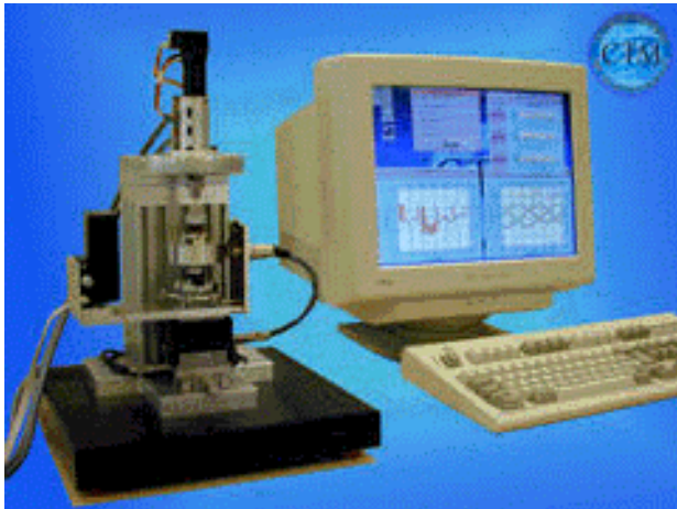
Figure 5: Micro torque testing stage
