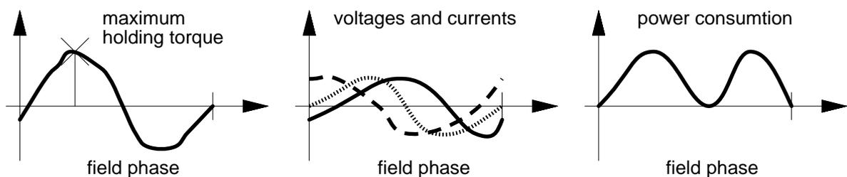
Figure 3: Torque-field phase characteristics of a stepper motor.
