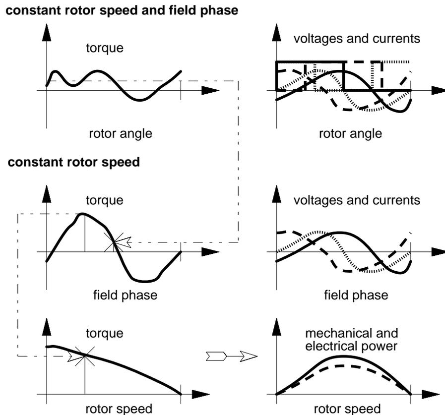
Figure 4: Torque-speed characteristics of a synchronous motor.
