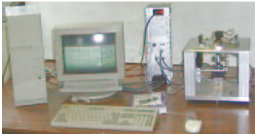
Fig. 1: Micro torque testing stage with its mechanics (right), electronics (middle) and the computer (at this time a 486/33).
